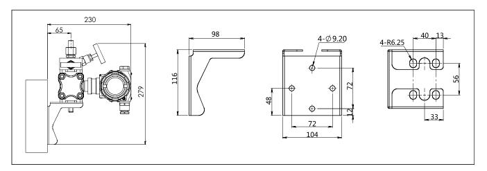
Pipe mounting flat bracket (B3)drawing and dimension (unit:mm)
